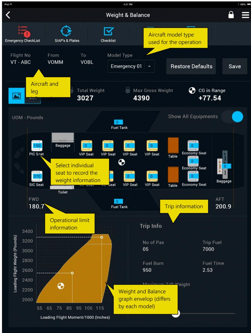
The Pilot can tap on the respective seat and the pop-out (refer image below) appears from which the Pilot will be able to ensure the seat is active in condition, Drop is applicable or not and weight information for the pax.
